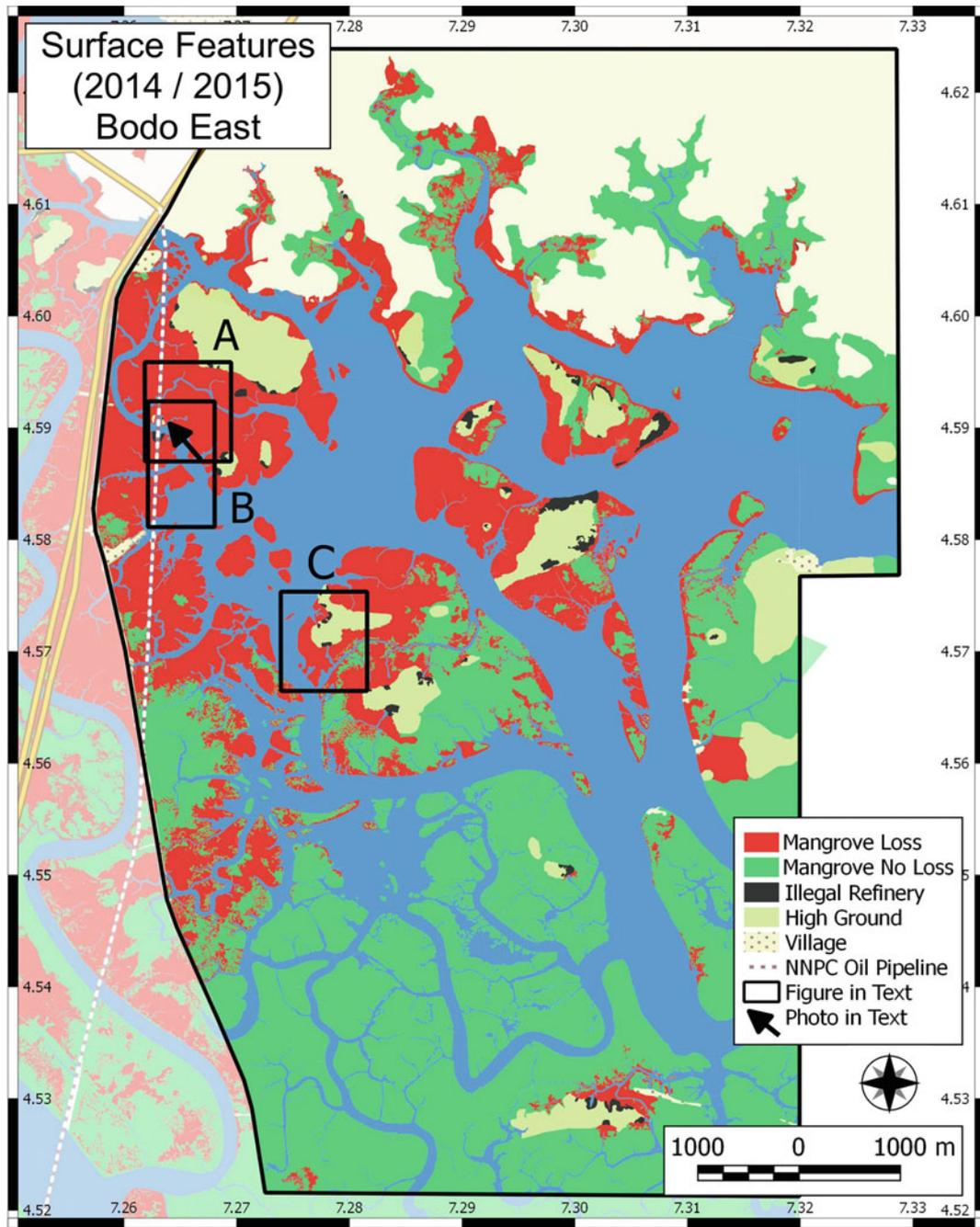
**Fig. 13.35** Bodo East surface features and mangrove loss. Areas shown as 'A', 'B' and 'C' are discussed further in the text
