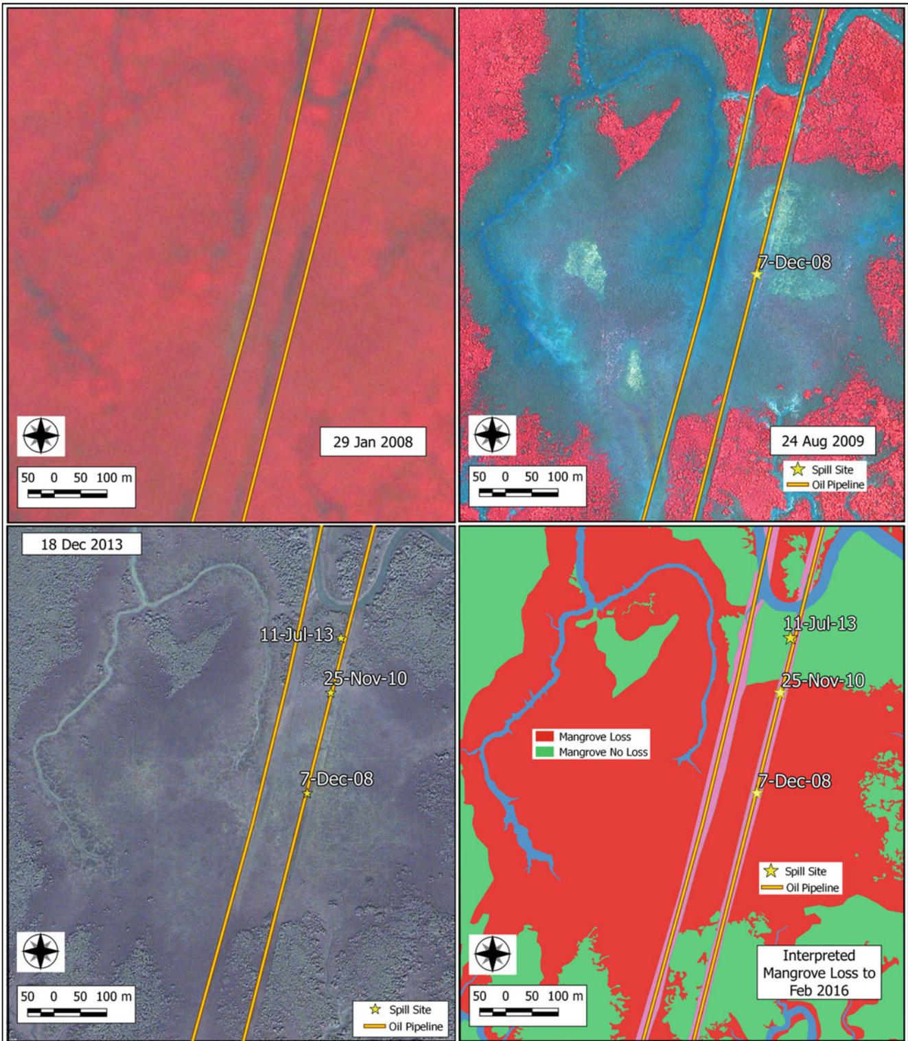
**Fig. 13.30** Bodo West area 'B' sequence of mangrove loss 2008–2013, attributable to the 7 December 2008 oil spill. Additional images from Google Earth 2013 to Feb 2016 show mangrove losses remain similar to that in 2013. Figure 13.25 shows the site location
