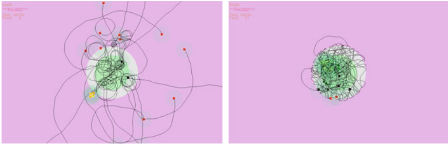
Fig. 4 Kilobot trails from simulation of the fittest controller in the first generation (left) and the 200th generation (right) of the fittest lineage
