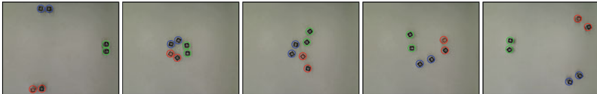
Fig. 8 Execution of the proposed algorithm in a scenario with 6 e-puck robots distributed in 3 groups
