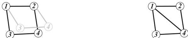
(a) A flexible framework with another (gray) incongruent embedding satisfying the distance function. (b) Adding the edge 14 results in a minimally rigid framework.
