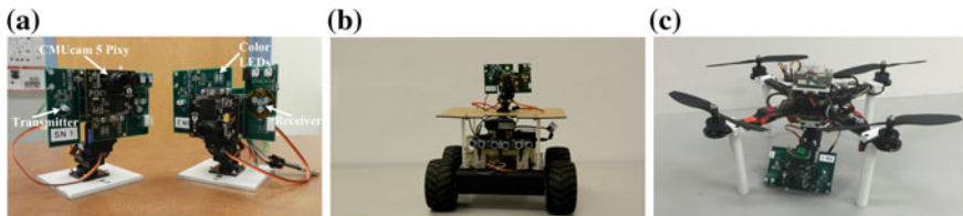
Fig. 4 a OW transceiver prototypes. OW transceiver mounted in b a Swarmie mobile ground robot, and c an AscTec hummingbird quadrotor
