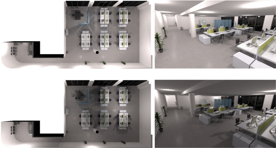
Fig. 3. Two renderings, a plan view and an interior view, of two different optimal light configurations in the open-space office.
