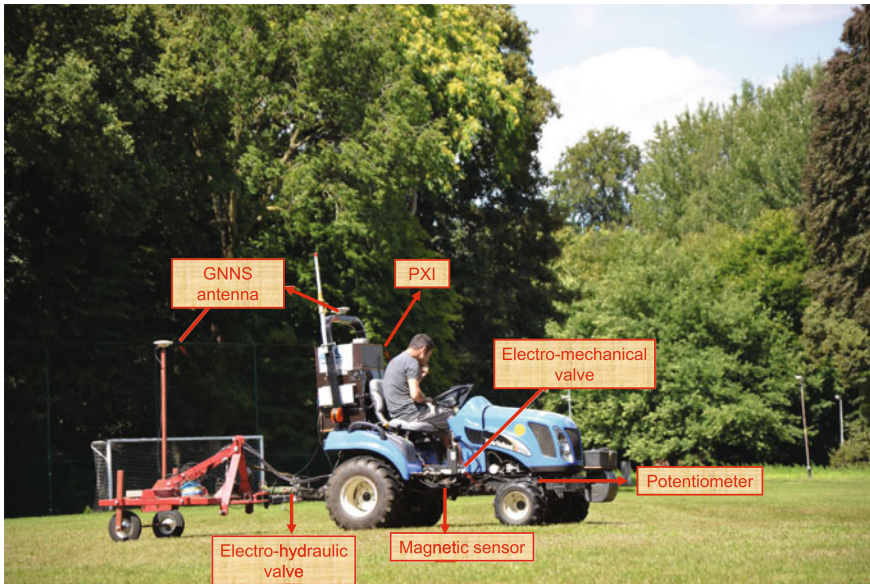
Fig. 1 The tractor-trailer system
