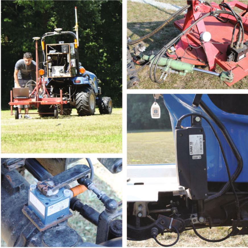
Fig. 2 Trailer actuator (top right), potentiometer (bottom left) and hydrostat spindle actuator (bottom right)
