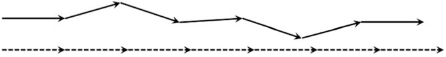
Fig. 7.1 Schematic of a vector mean (above) and a scalar mean (below). All single vectors have equal length, but the direction is changing slightly in the vector mean example. The mean is a vector pointing from the end of the first vector to the tip of the last vector and whose length is divided by the number of vectors involved in the mean
