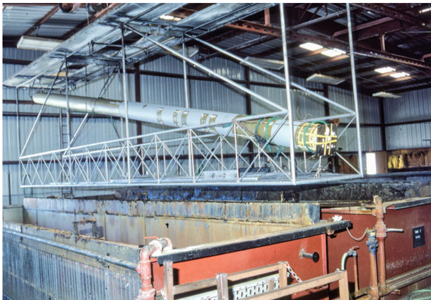
Fig. 11 Cross beam for “stars and stripes ’88” being chemical milled to reduce wall thickness
