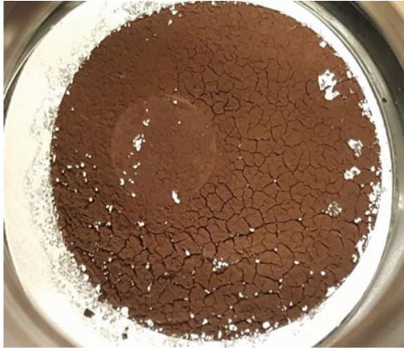
Fig. 2 Filtered copper coated CNT's of a brown color
