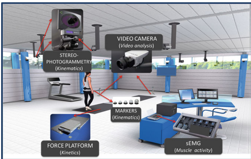
Fig. 1 Typical equipment of a Gait Analysis Lab
