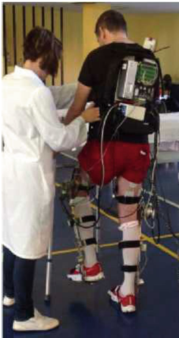
Fig. 4 Patient with incomplete spinal cord injury walking with the hybrid FES-powered exoskeleton Kinesis [92]
