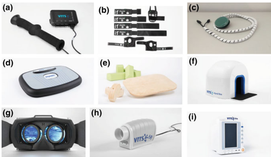
Fig. 2 A number of technological components and devices expand the capabilities of the VRRS, e.g. magnetic-based and IMU-based tracking systems, together with wearable bands and textiles to apply sensors to the patient's body (a, b, c); posturographic and proprioceptive boards (d, e); a camera-based tracking system for the hand (f); virtual reality headsets (g); and systems for tracking cardiorespiratory parameters and respiratory patterns (h, i)
