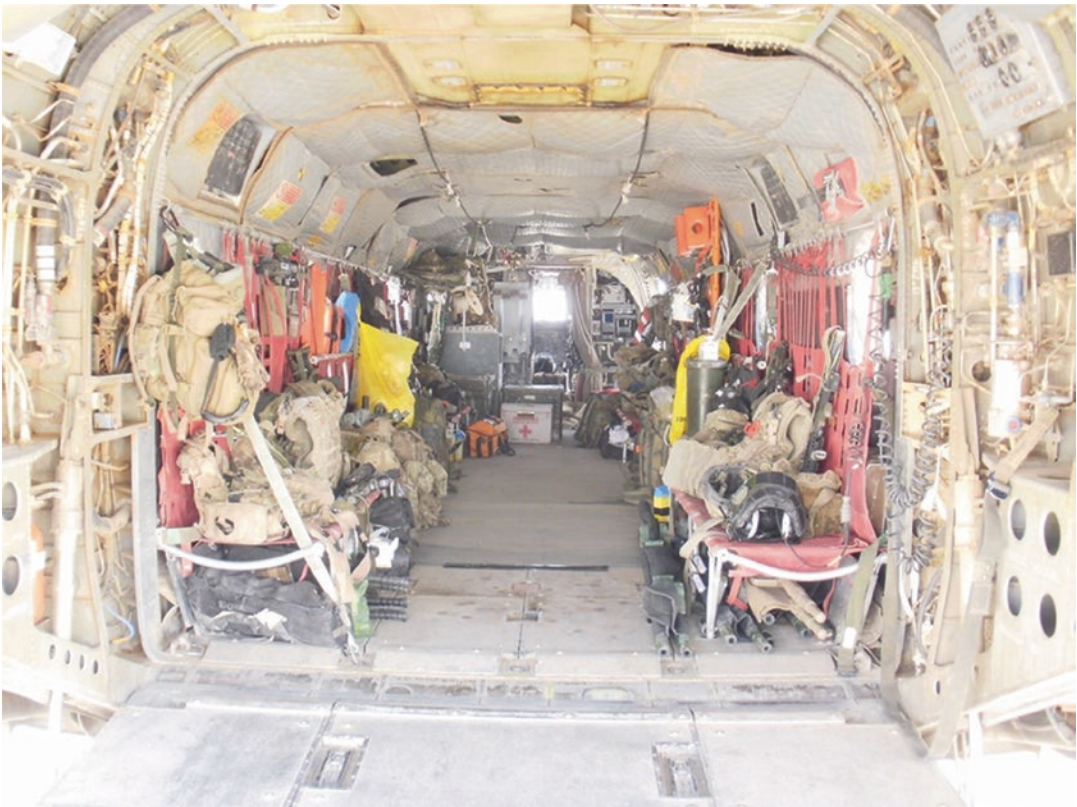
Fig. 6.1 A CH-47 Chinook helicopter being used for prehospital casualty retrieval. The floor space allows all-round access to litter patients, and the aircraft is large
