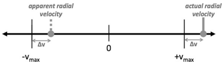
Fig. 10 Schematic illustrating Doppler velocity aliasing. If the true radial velocity (gray line) exceeds the magnitude of the Nyquist velocity ( \pm v_{max} ), then the radar interprets the apparent radial velocity (dashed gray line). Note that in this case the aliased Doppler velocity is of opposite sign to the actual radial velocity
