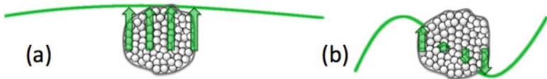
Fig. 2 Schematic showing (a) a particle small compared the wavelength (traced out by the green line) in which the electric field (green vectors) is uniform throughout the particle, and (b) a particle large compared to the wavelength in which the electric field is nonuniform throughout the particle. In (a), the induced dipoles oscillate in phase with one another. In (b), the induced dipoles oscillate out of phase with one another
