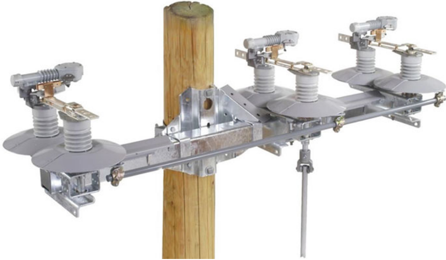
Fig. 2.48 29 kV, 900 A, 25 kA one-second short time and 42 kA peak fault closing. (Courtesy of S&C Electric Company)
