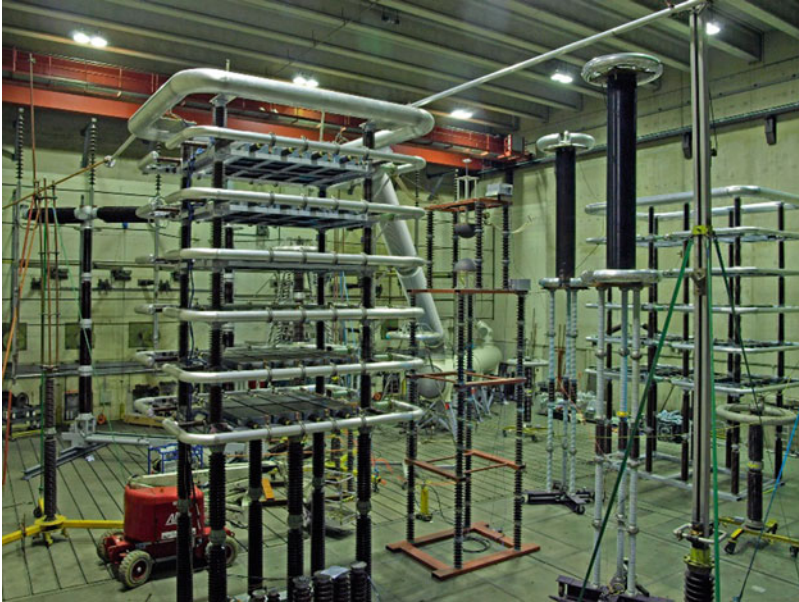
Fig. 11.23 Setup at KEMA Laboratories for full-pole short-circuit tests of a 1100/1200 kV circuit breaker. (Courtesy of DNV GL KEMA Laboratories)
