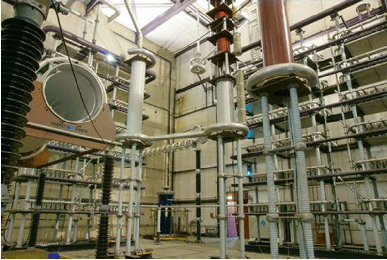
Fig. 11.15 Photo of (part of) a synthetic voltage source for producing (T)RV in HV circuit-breaker tests. (Courtesy of DNV GL/KEMA Laboratories)
