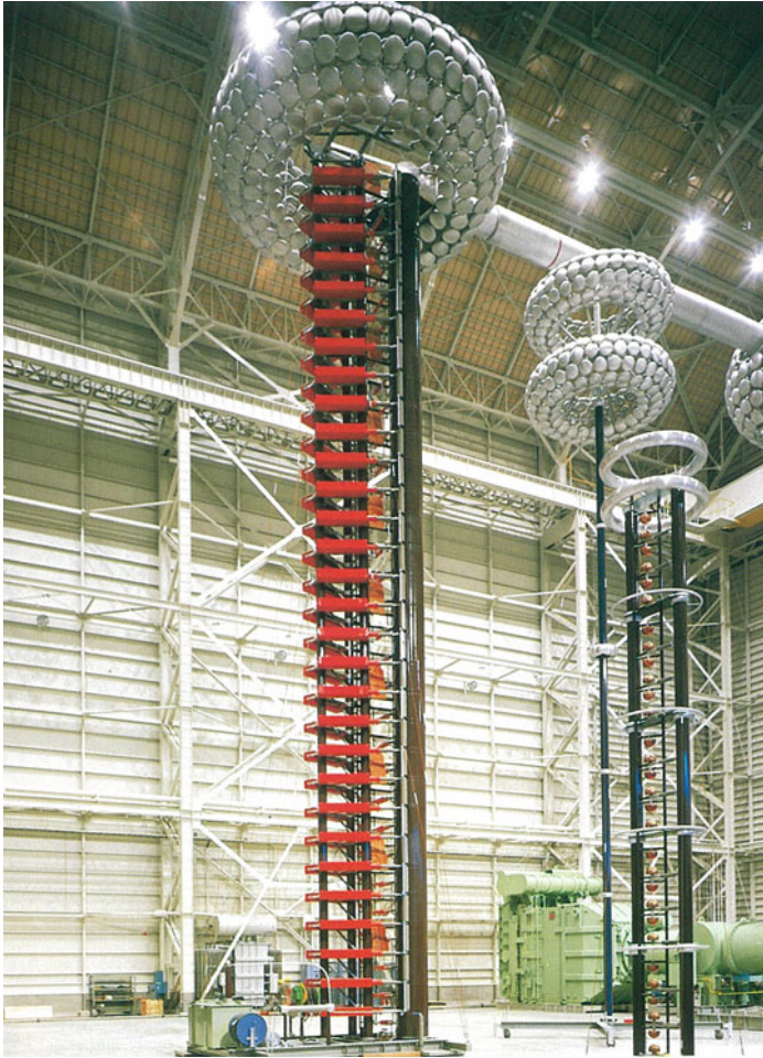
Fig. 10.9 A photo of 6000 kV, 450 kW impulse voltage generator. (Courtesy of Mitsubishi Electric)
