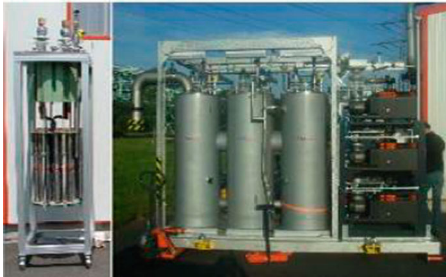
Fig. 13.19 A 12 kV, 800 A SFCL
