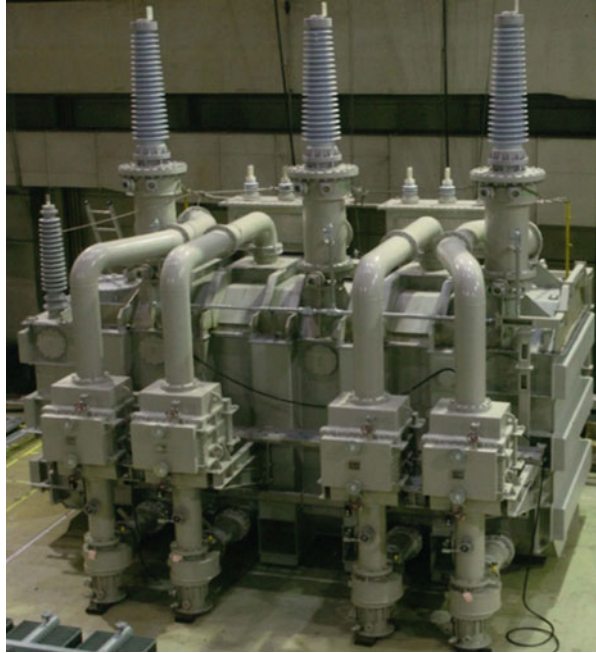
Fig. 2.20 132 kV 50 MVA SF 6 gas-insulated power transformer (core type)
