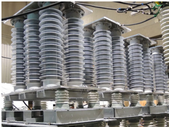
Fig. 15.10 Example of multicolumn MOSA units for prototype HVDC circuit breaker. (Energy dissipating capacity: 4 MJ)
