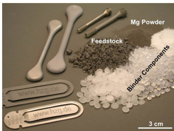
Fig. 1 Mg-alloy demonstrator parts and test specimens made by MIM of Mg at Helmholtz-Zentrum Geesthacht
