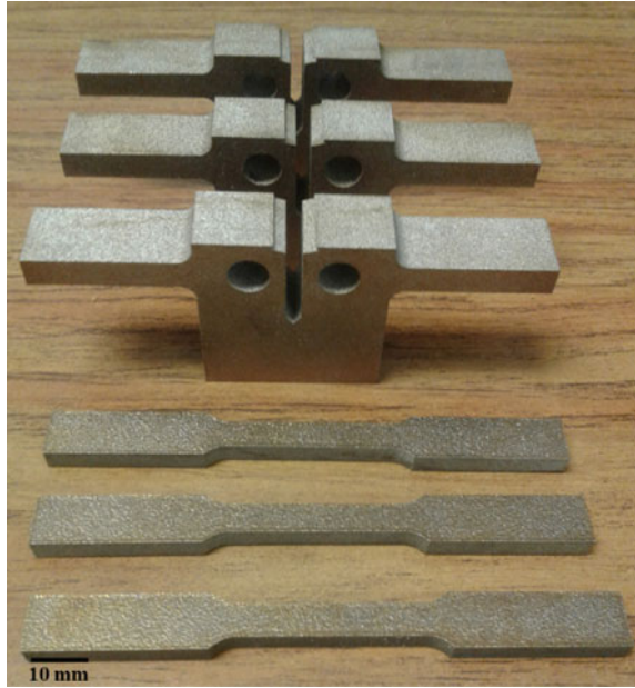
Fig. 1 A typical batch of tensile and fracture toughness specimens produced by DMLS
