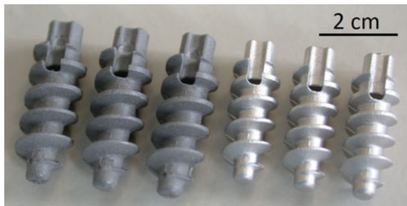
Fig. 9 Suture anchor implant screw demonstrator part made by MIM of EZK400 material. Design: ConMed, USA
