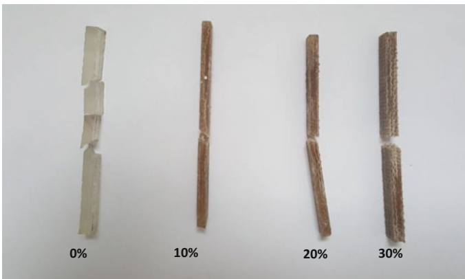
Fig. 3 Typical macrostructural aspects of flexural specimens of polyester composites reinforced with different volume fractions of jute fabric
