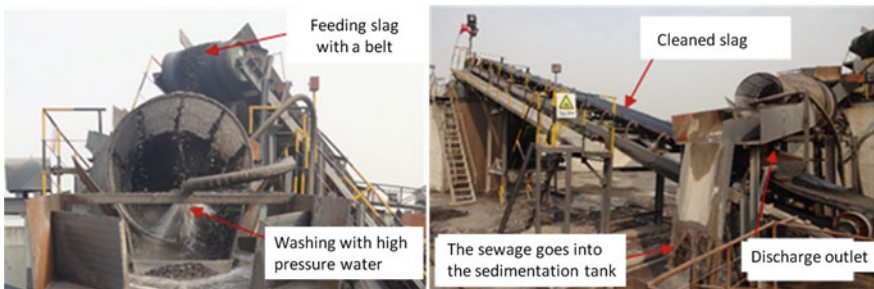
Fig. 9 Cleaning technology of BOF slag aggregate
