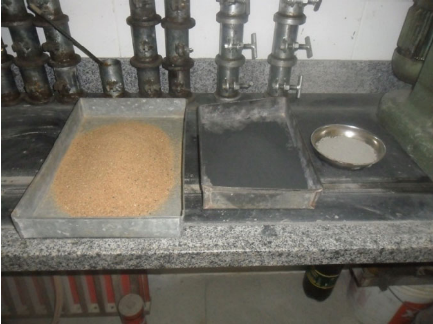
Fig. 1 Sand, dregs, and cement for the confection of the mortar, respectively
