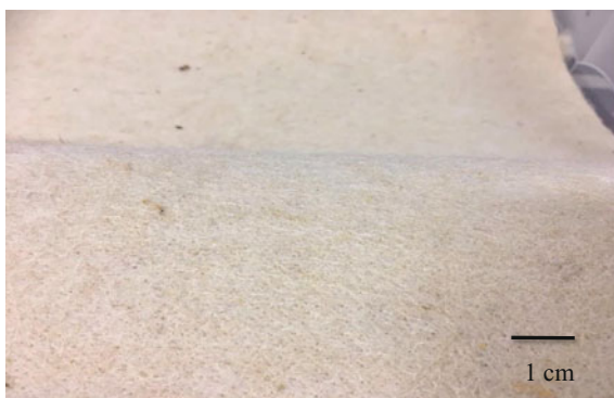
Fig. 1 The 70% malva /30% jute hybrid blanket
