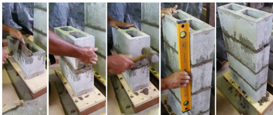
Fig. 2 Four-block prisms production
