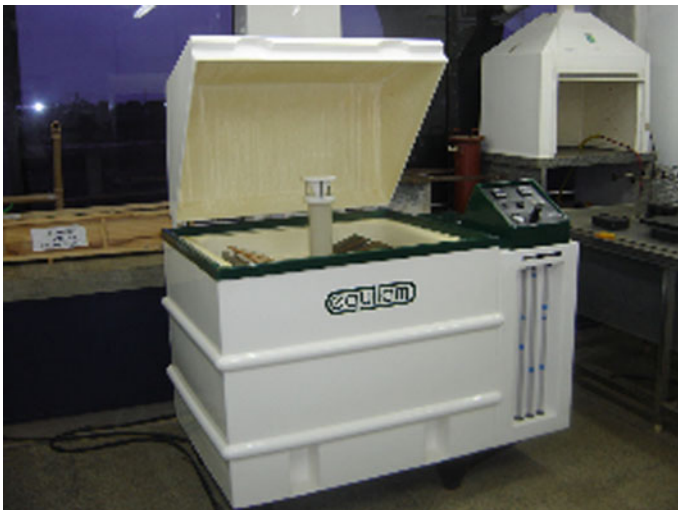
Fig. 2 Salt spray equipment. Source own author
