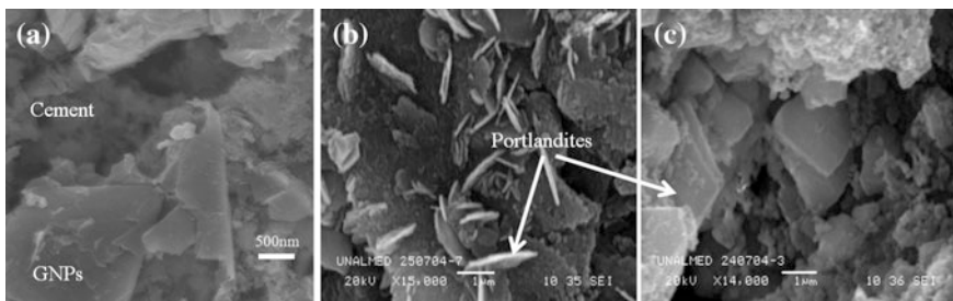
Fig. 4 Images taken with transmission electron microscopy (TEM)) for a reinforced concrete with graphite nanoplatelets (GNPs), b and c the nanostructure Portland cement phase portlandite
