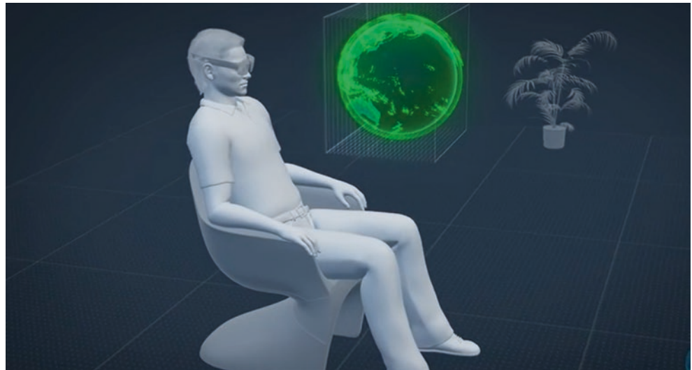
Fig. 44.2 The same object in Fig. 44.1 is projected as a hologram that occupies 3D space, as opposed to one single focal plane. The fixed coordinates and multiple focal planes afford interaction with and within the image at arm's reach of the observer
