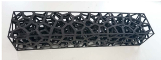
Fig. 27.1 A sample structure fabricated by use of 3-D printer. The volume fraction of the substantial portion is about 10%, and it is easily controlled by setting the thickness of line segments of Voronoi polyhedra.
