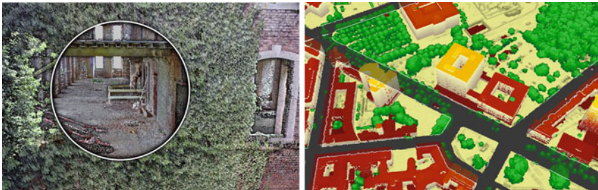
Fig. 2.6 Focus + context visualization for massive point clouds. Left: Using an interactive see-through lens, the occluded interior of a building can be inspected in the context of the overall scan. Right: A visibility mask is used to highlight otherwise hidden street points
