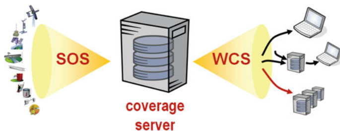
Fig. 14.15 OGC service pipelines: upstream SOS and downstream WCS
