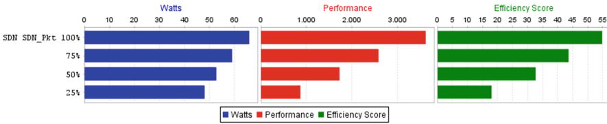
Fig. 5. Example result from an energy efficiency measurement with four load levels
