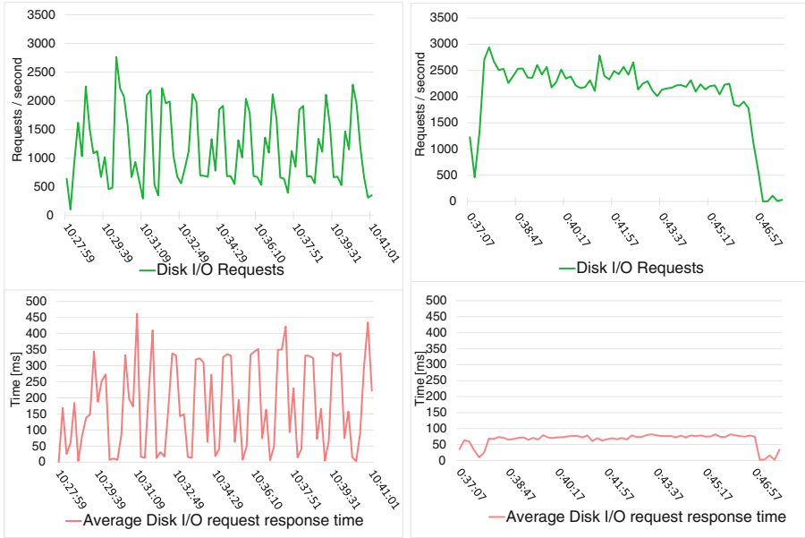
Fig. 3. Disk traffic for a 130 GB Naive Bayes workload (left: ARM, right: x86).
