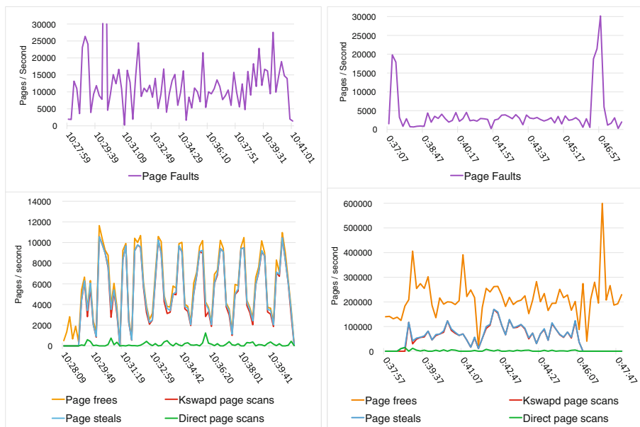
Fig. 5. Memory management for a 130 GB Naive Bayes workload (left: ARM, right: x86). Note the difference in y-axis scales in the bottom graphs.
