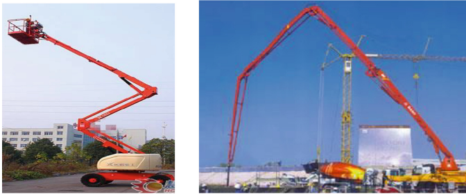
Fig. 1. Flexible arms in real life: hydraulic aerial cage (left) and concrete pump truck (right).
