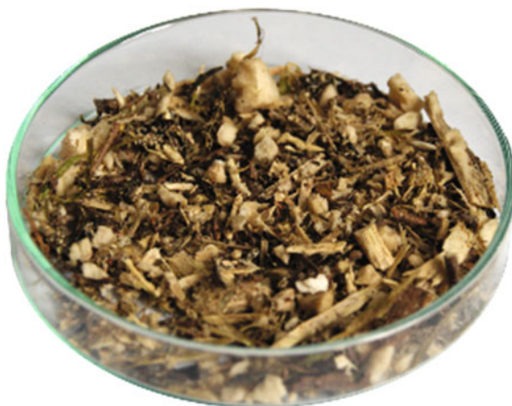
Fig. 2 Raw black lilac chips after the plant had been cut and shredded
