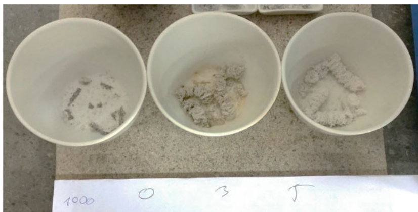
Fig. 3 View of the sample ashes at 1000 °C. From left samples with 0; 3 and 5% kaolinite content, sulfur content in all samples 2%
