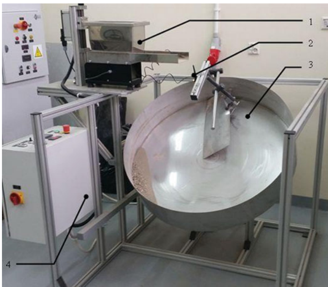
Fig. 2 GitTech Disc Granulator; 1 vibrating material dispenser, 2 spray nozzles granulate material, 3 the plate on which the granulation process takes place, 4 control panel
