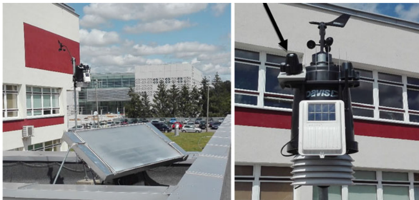
Fig. 4 SAH tested experimentally in normal operating conditions (left) and the weather station view (right), the solar irradiation sensor inclination was set just like the SAH one
