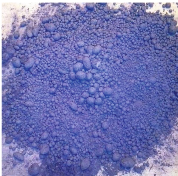
Fig. 5 Granule sample A1 code obtained on a disk granulator
