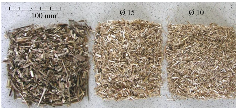
Fig. 2 Shredded Mushroom Shoots: from the right grinded on the ax cutter, then ground on a mill with Ø15 mm and Ø10 mm sieve Source Own elaboration
