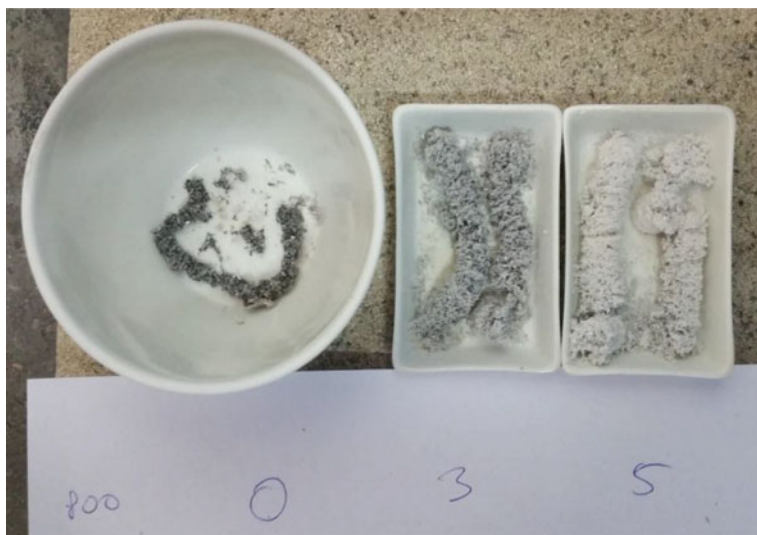
Fig. 2 View of the sample ashes at 900 °C. From left samples with 0; 3 and 5% kaolinite content, sulfur content in all samples 2%
