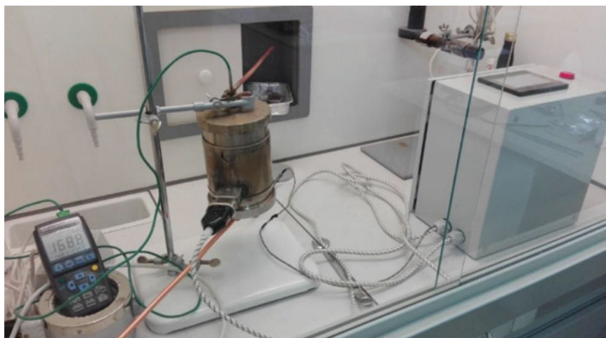
Fig. 2 Laboratory scale pyrolysis stand
