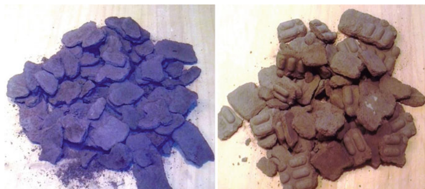
Fig. 4 Granulate A1 obtained from cylindrical compactor; from the left with smooth rollers, then using a smooth roll cooperating with a roll with recesses
