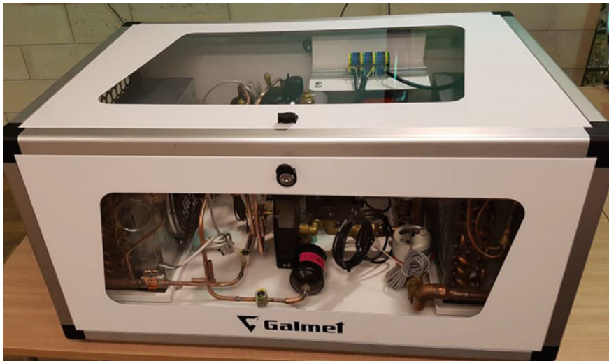
Fig. 2 Didactic air–water type heat pump. A heat pump with temperature stabilization on the side of the heat source and heating system
