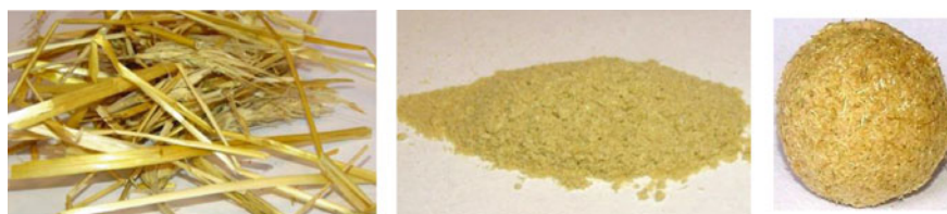
Fig. 3 Raw wheat straw (a), sawdust (b) and spherical pellet (c) ( d = 10 \text{ mm} )
