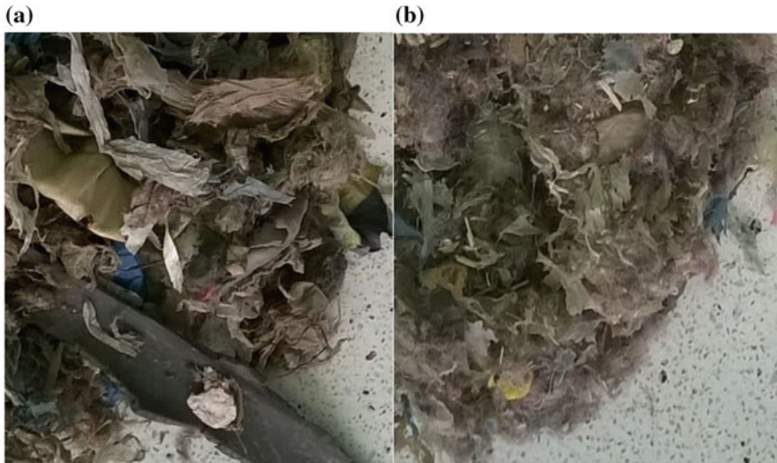
Fig. 1 Raw material: a after delivery from RIPOK, b after milling (diameter of sieve 15 mm)
