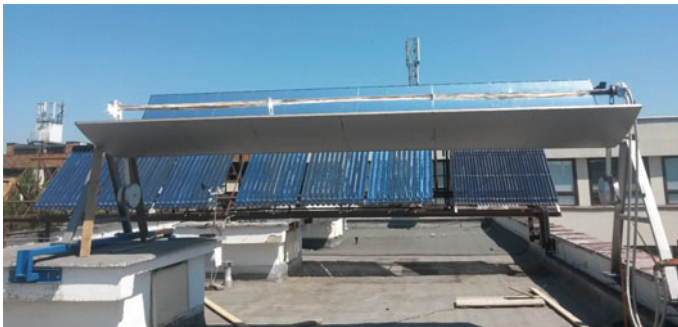
Fig. 2 Parabolic trough collector with one-axis tracking
