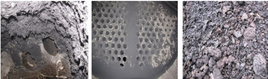
Fig. 3 Problems with low temperature melting behavior of ash
