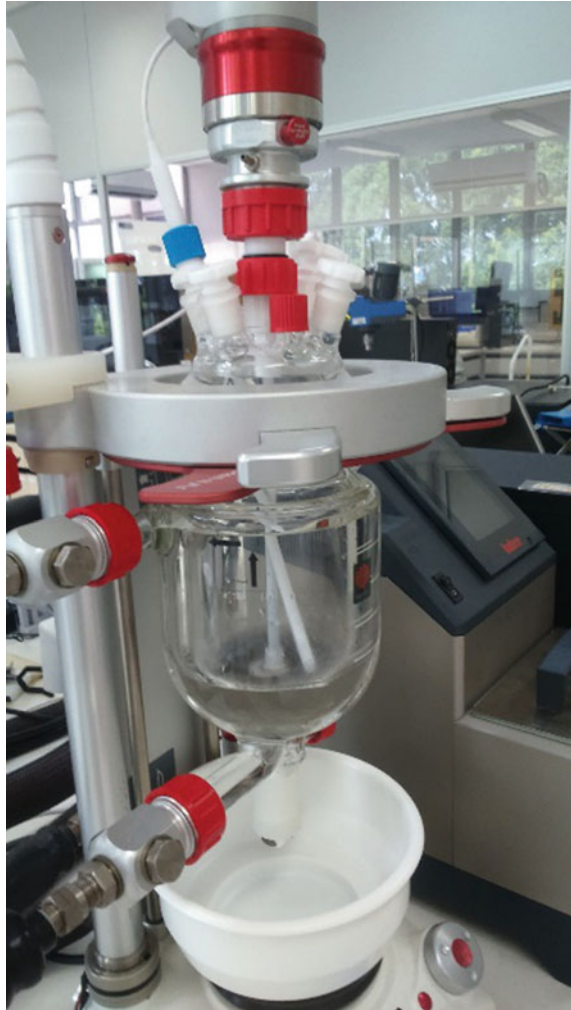
Fig. 2 Jacketed reactor used for leaching of indium from a-Si module
