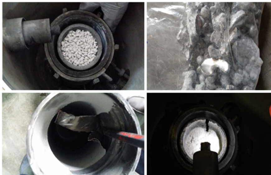
Fig. 3 Comprehensive experimental raw materials and products. (Left upper: pellet; left lower: crystalline magnesium; Right upper: nickel-iron alloy; right lower: slag)
