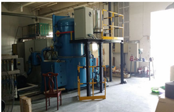
Fig. 2 120 kW serpentine continuous reduction of magnesium test furnace
