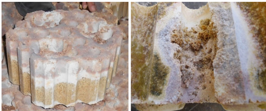
Fig. 8 Erosion of upper silicon checker brick in hot blast stove
