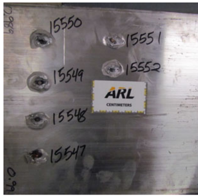
Entry of Impact - 25.4-mm x 304.8-mm (1-inch x 12-inch) AMX602-T1 plate
