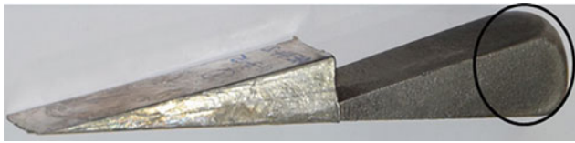
Fig. 2 Alloy was cast into two-part wedge shaped moulds consisting of a permanent metal mould (left) and a sand mould (right)
