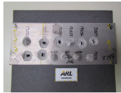
Exit of Impact - 25.4mm x 152.4mm (1-inch x 6-inch)
