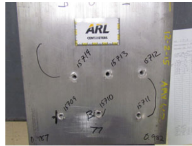
Entry of Impact - 25.4mm x 304.8-mm (1-inch x 12-inch)
