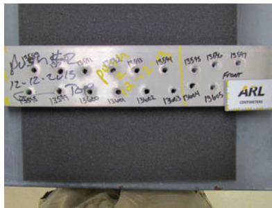
Entry of Impact - 25.4-mm x 101.6-mm (1-inch x 4-inch)
