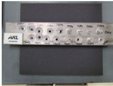
Exit of Impact - 25.4-mm x 101.6-mm (1-inch x 4-inch)
