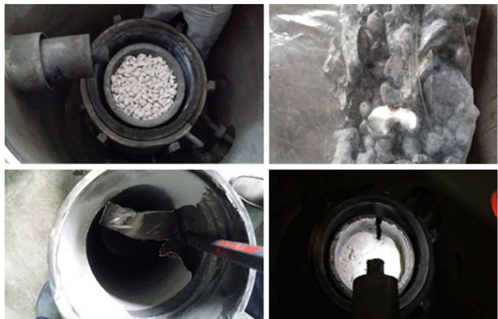
Fig. 5 Comprehensive experimental raw materials and products left upper: pellet; left lower: crystalline magnesium; right upper: nickel-iron alloy; right lower: slag
