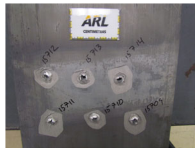
Exit of Impact - 25.4mm x 304.8-mm (1-inch x 12-inch)
