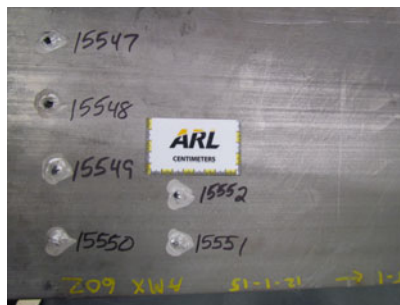
Exit of Impact - 25.4-mm x 304.8-mm (1-inch x 12-inch) AMX602-T1 plate
