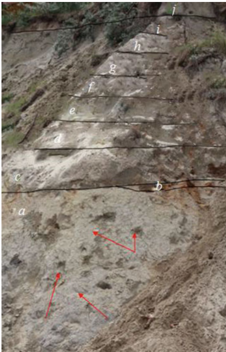
Fig. 2 Observation site 2. The bottom of the picture shows bluish dark-grey boulder sandy clay of the Early Baltic stage with cobble and gravel inclusions (indicated with red arrows ). It is followed by gravel and cobble deposits and interleaving fine sands of different colours containing glauconite
