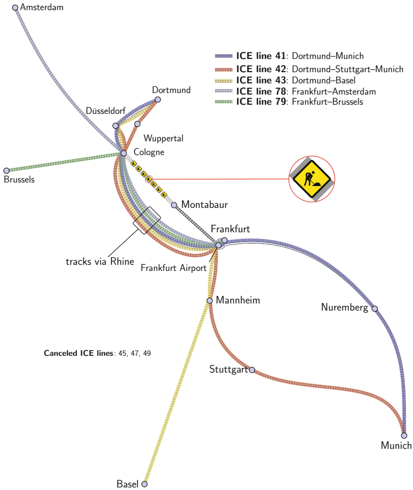
Fig. 10.3: Redirection for the Köln-Rhein-Main construction site (KRM): All ICE lines between Montabaur and Cologne were closed in order to rebuild rails (as indicated by the sleepers without rails) on four succeeding weekends in May 2015. Note that the figure only illustrates the situation at the weekend when the KRM is performed, i.e., the ICE lines 41, 42, 43, 45, 47, 49, 78, 79, and 82 operate as usual on the high-speed tracks between Frankfurt and Cologne from Monday to Friday. Note also that the placement of the locations is true to scale
