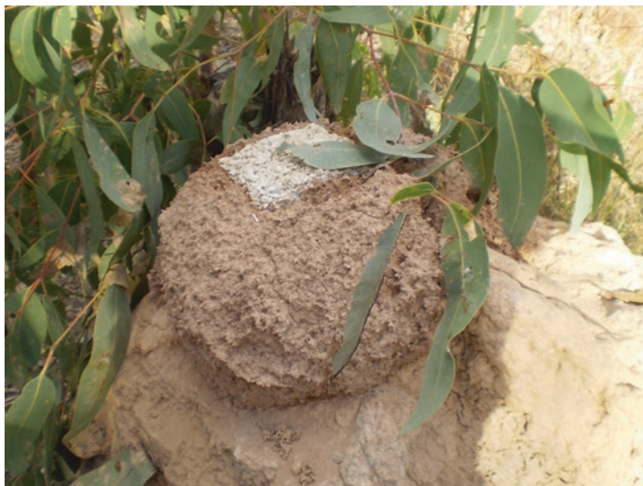
Fig. 9.1 Visible new soil deposition transported overnight around an intrusive section of hempcrete inserted into the top of the above-ground termite mound of Coptotermes acinaciformis in the Northern Territory (J.R.J French, personal communication)
