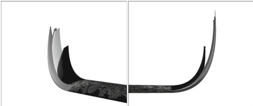
**Fig. 8.8** Winglet design iterations (0 = Initial, 10, 15, 19 = last design)
