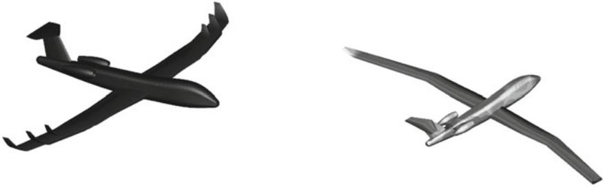
**Fig. 8.17** Wing + winglet MDO - design iterations and pressure distribution of final design
