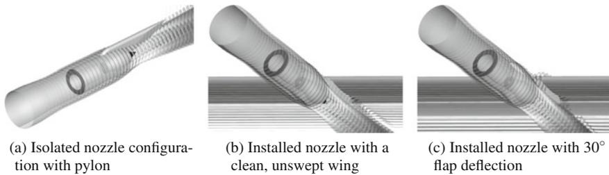
**Fig. 11.1** Overview of the VITAL BPR9 configurations employed for the TAU validation studies
