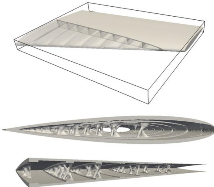
**Fig. 14.4** Topological optimization with an interior rib structure. Initial iteration (top) and two different cuts through the optimal solution (middle and bottom)
