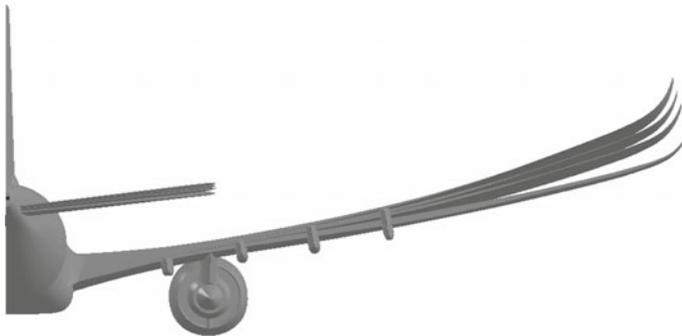
**Fig. 5.2** Illustration of changes in wing bend and HTP setting variations
