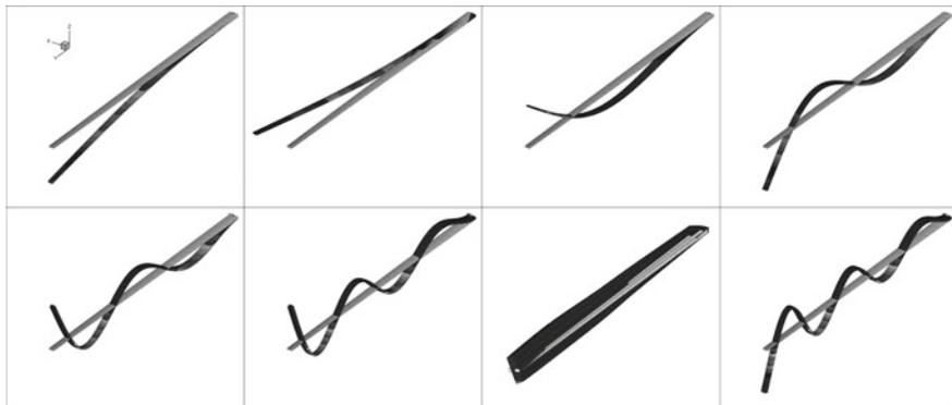
**Fig. 17.3** Selected normal mode shapes of the wing box test case (corresponding eigenvalues are given in Table 17.1)
