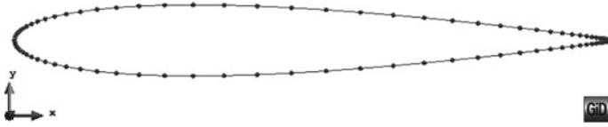
Fig. 9.10 The design mesh of the NACA0012 airfoil
