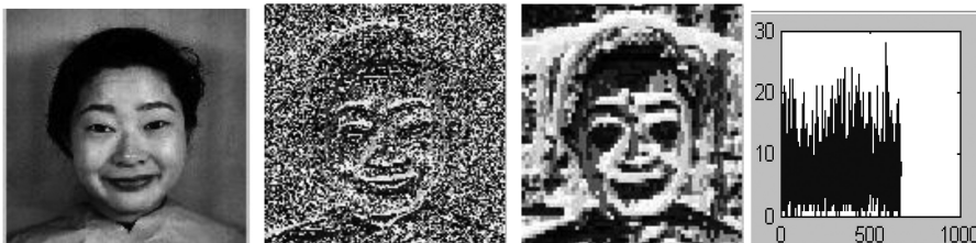
Fig. 2. Original image, LBP image, Wavelet + new LBP image and Histogram of the new LBP image
