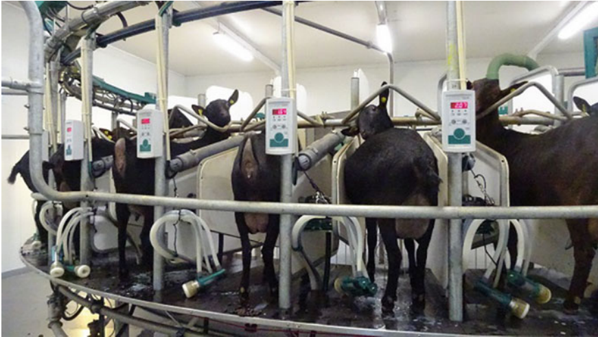
Fig. 19.1 Rotary (carousel) radial milking machine with 32 places. At the end of milking, the teat cups detach automatically from teats preventing long milking duration and consequently potential udder damage (Besier et al. 2016) (provided by J. Simões)
