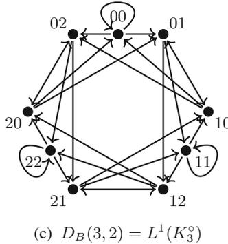
**Figure 11.5** Construction of a Kautz digraph via the line digraph operator or from a de Bruijn digraph.
