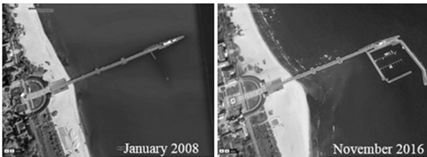
Fig. 1 Changes in the shoreline near the Sopot Pier (left side: January 2008, right side: November 2016) Google earth V 7.1.8.3036
