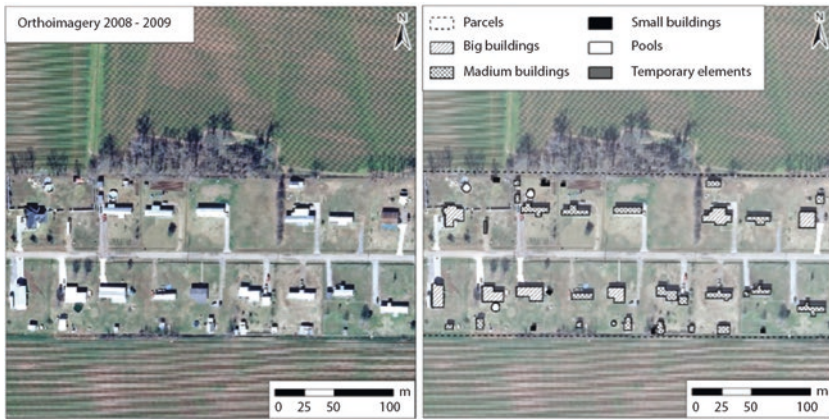
Fig. 2.5 Orthoimage of 2008–2009 of an area of residential development within the West Atchafalaya Floodway ( left ) and same view with various types of encroachments identified ( right ), at coordinates 91^{\circ}50'9.288''\text{W} and 30^{\circ}59'13.533''\text{N} (Source: US Geological Survey; accessed at earthexplorer.usgs.gov , used by permission)
