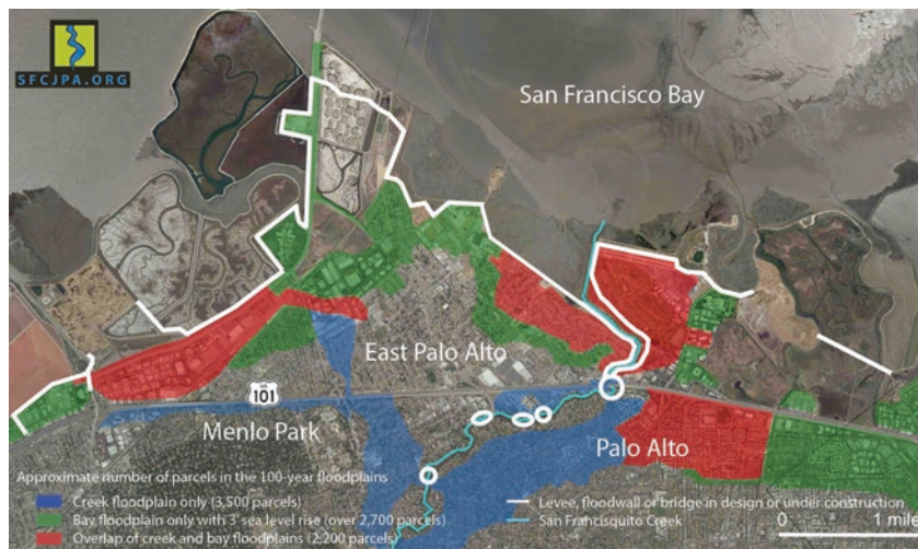
Fig. 5.6 San Francisquito Creek Area projects and floodplains (Courtesy of San Francisquito Creek Joint Powers Authority, 2017)
