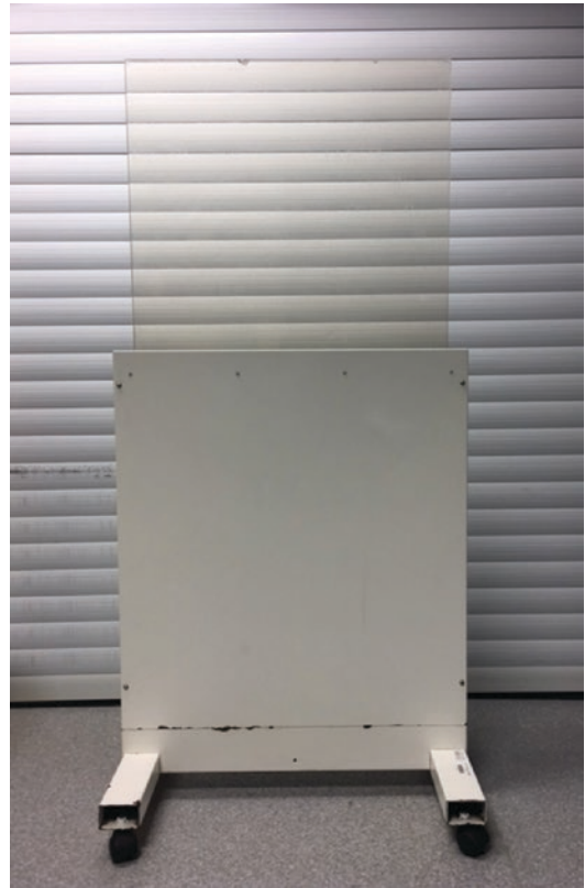
Fig. 7.3 Mobile protective shielding. This protective shield has wheels to allow mobility and a transparent leaded screen for visualization. This allows catheter laboratory staff added protection. However full-body radiation protection must still be worn
