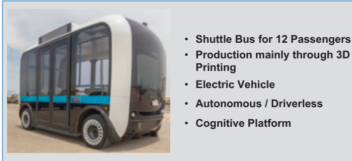
Fig. 9.11 Electrically powered, autonomously driving shuttle bus (according to [Mol16])
