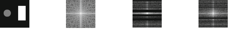
Fig. 2. (a) f(x) ; (b) Frequency function \log(|\hat{f}(\omega)|) after shifting; (c) and (d) Sampling noisy frequency data P_{60}\log(|\hat{g}^\delta(\omega)|) and P_{90}\log(|\hat{g}^\delta(\omega)|) after shifting.
