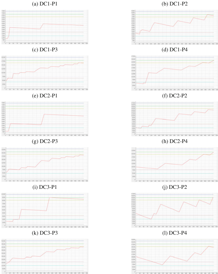
Fig. 16.4 Inventory graphics of every pair DC-product. Where the X-axis is the considered horizon in hours (from 0 to 525 h) and Y-axis is the volume in m^3 . The red line represents the inventory at each moment; the dark blue line is the physical capacity level; the outer intermediary lines are the maximum and minimum level; and the inner intermediary lines are the maximum and minimum target level
