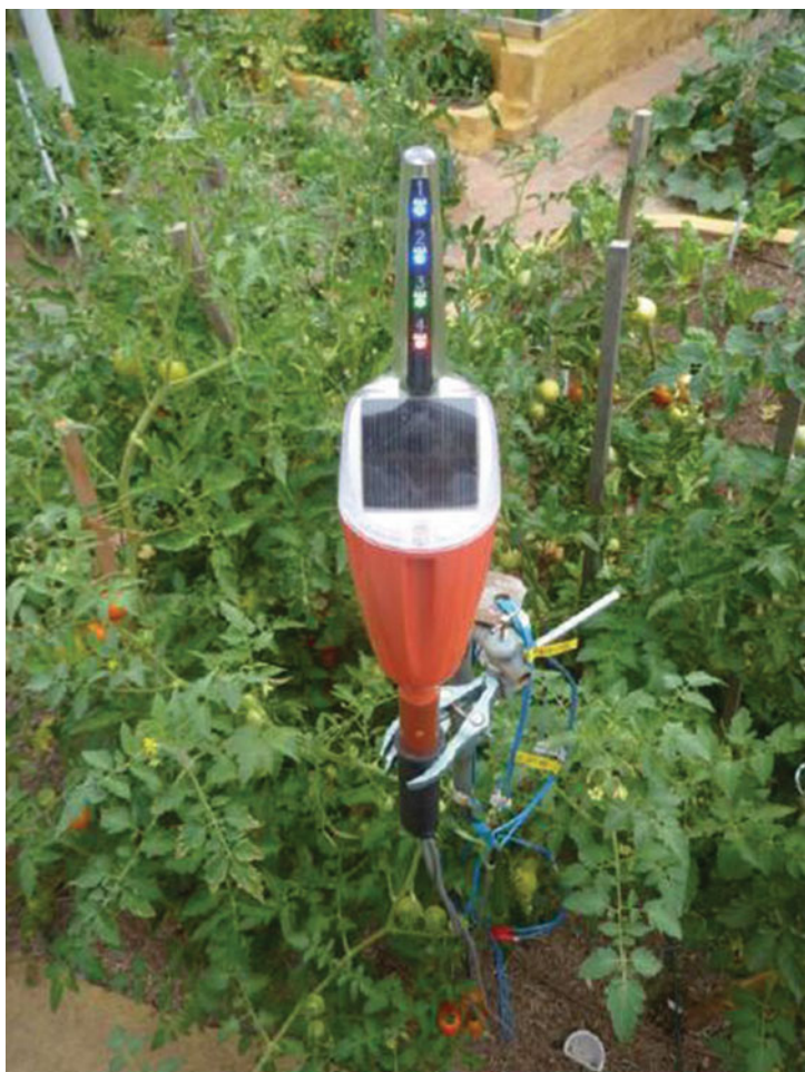
Plate 9.1 Chameleon sensors (blue wires) buried below the soil surface in a tomato crop field and connected to the solar-powered chameleon reader with different colours (blue, green, red). Picture by Ikenna Mbakwe (2014)
