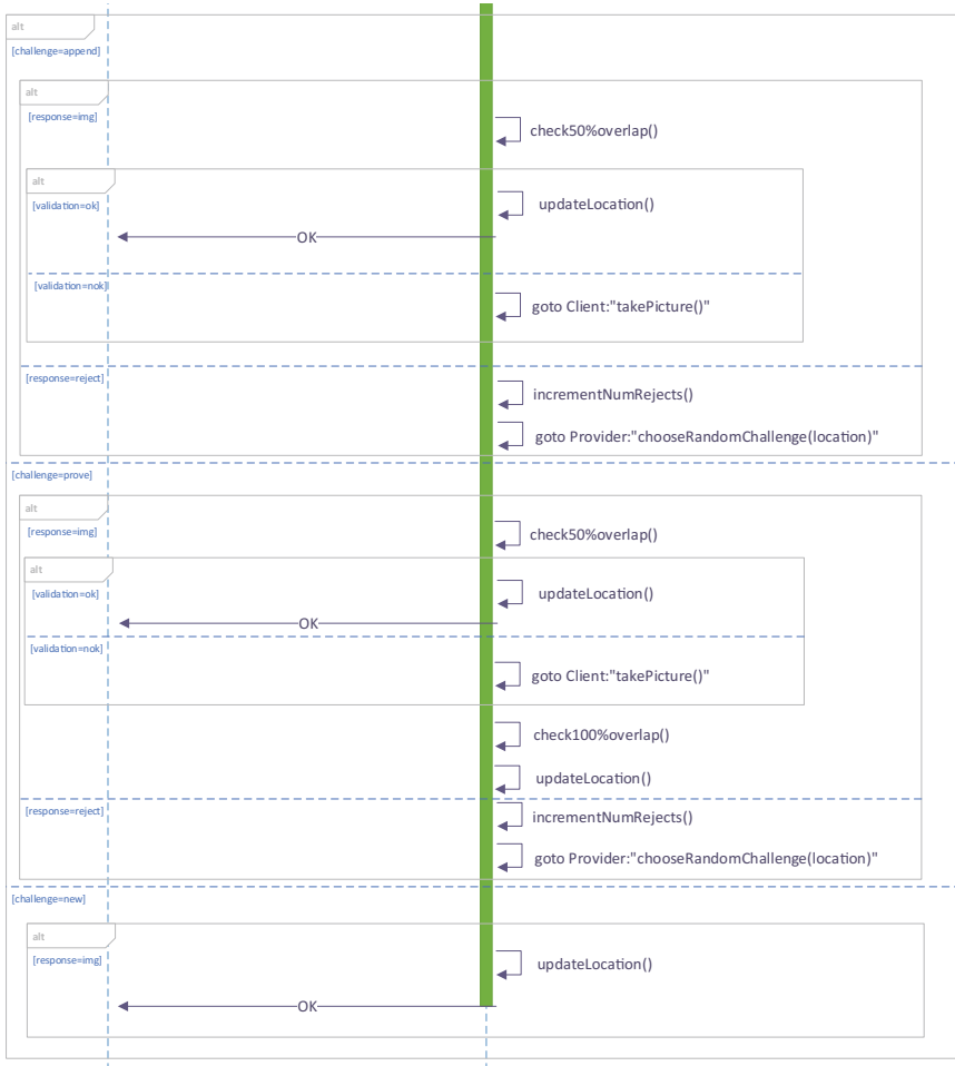
Fig. 7 An UML sequence diagram depicting the “The Reaction” step of the CLP procedure
