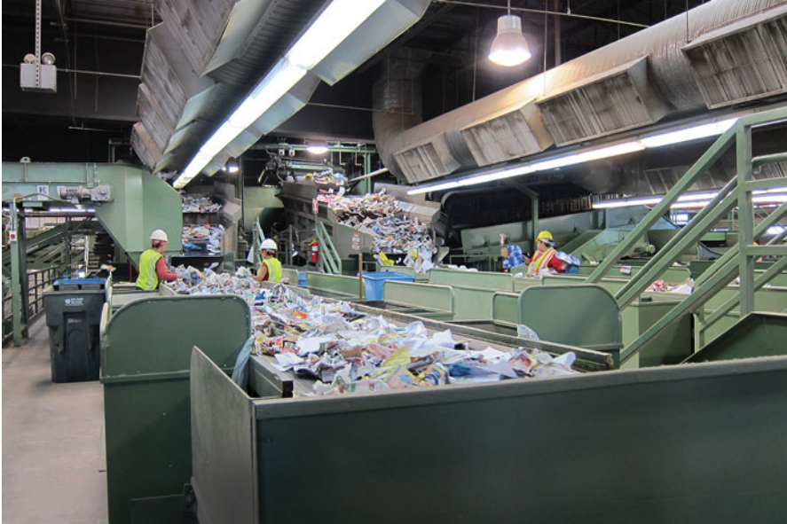
Fig. 3 Phoenix Public Works workers sorts through paper waste at the 27th Avenue Waste Transfer Station for bundling into recyclables and reusables. Feedstocks like this will be available to companies based at the Resource Innovation Campus and RISN Incubator (Photo courtesy of City of Phoenix Public Works Department)
