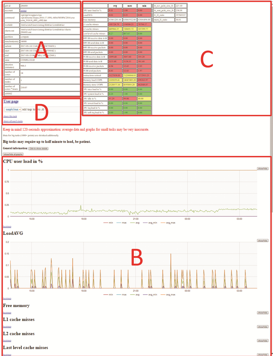
Fig. 2. JobDigest report blocks: A – general job information, B – dynamic job characteristics, C – integral job characteristics, D – tags and job categories.
