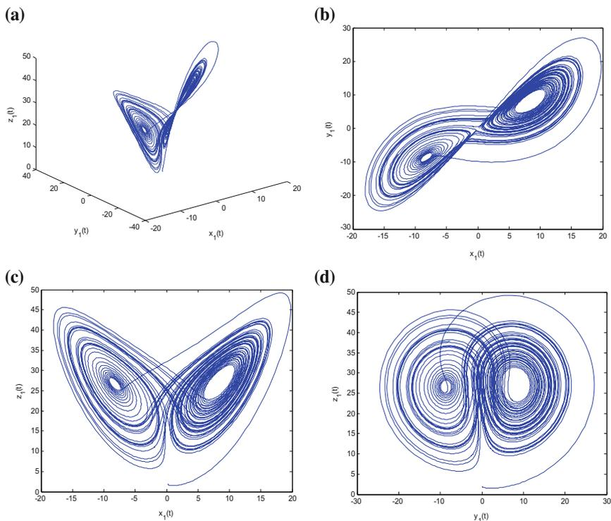
**Fig. 2** Phase portraits of the Lorenz system with uncertain parameters and external disturbances at  $q=0.993$ : **a**  $x_1 - y_1 - z_1$  space, **b**  $x_1 - y_1$  plane, **c**  $x_1 - z_1$  plane, **d**  $y_1 - z_1$  plane
