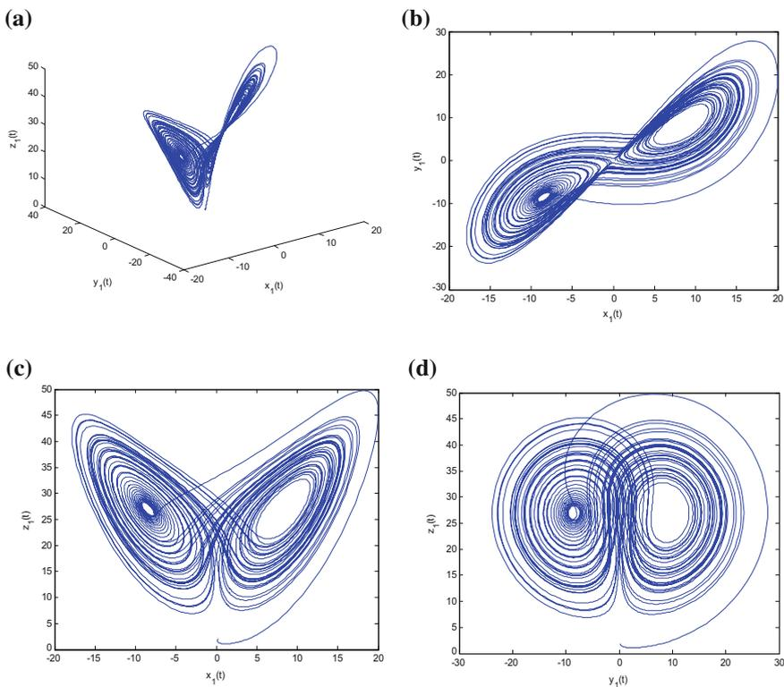
**Fig. 1** Phase portraits of the Lorenz system at  $q=0.993$ : **a**  $x_1 - y_1 - z_1$  space, **b**  $x_1 - y_1$  plane, **c**  $x_1 - z_1$  plane, **d**  $y_1 - z_1$  plane
