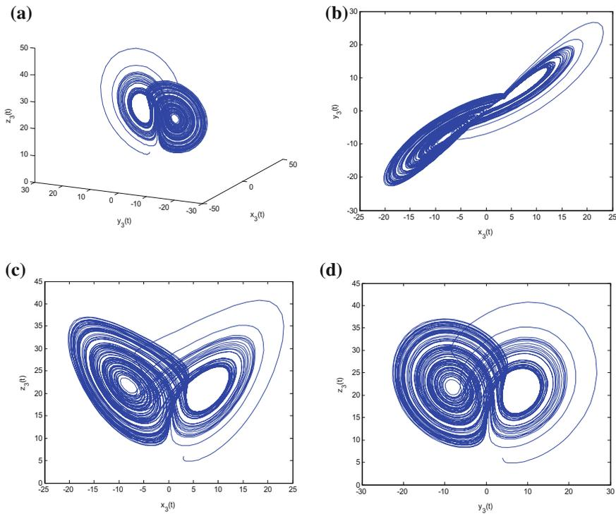
**Fig. 6** Phase portraits of the Chen system with uncertain parameters and external disturbances at  $q = 0.90$ : **a**  $x_3 - y_3 - z_3$  space, **b**  $x_3 - y_3$  plane, **c**  $x_3 - z_3$  plane, **d**  $y_3 - z_3$  plane
