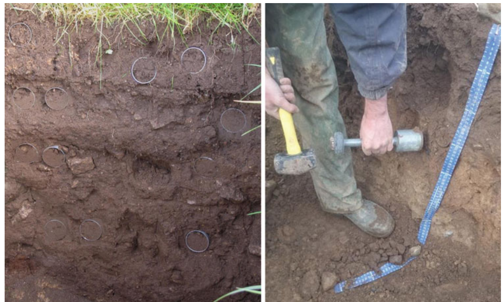
Fig. 3.4 Three bulk density rings per horizon as a physical soil measurement shown on left, method for bulk density measurements shown on right (Photo: Jeremy Emmet-Booth)
