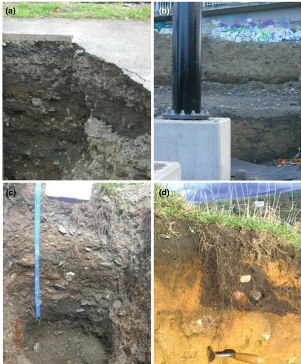
Fig. 3.11 Urban soils. a Ekranic Technosol, a pavement with constructed deposits below, formerly a tramline, road base, and embankment. b Regosol, formed during soil relocation as cut-and-fill for highway construction; this will eventually be given a topsoil cover and grass seed sown. c Garbic Technosol (Thapto-Fluvisolic), reclamation deposits of commercial garbage, with many artefacts such as bottles; beach sediments lie a further 80 cm below the base of this hand-dug pit. d Regosol (Relocatic), a reclamation deposit over a worked-out sand pit, showing remnants of former site soils, roughly mixed
