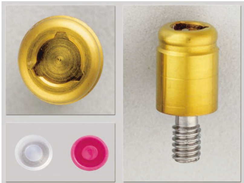
Fig. 11.12 Stud-type attachment system with a cylindrical-shaped male component displaying both extra- and intracoronal retentive characteristics and a female part comprised of nylon inserts in a metallic housing
