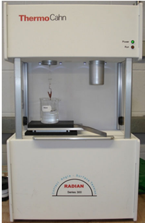
Fig. 2.18 Dynamic contact angle analyser test set-up
