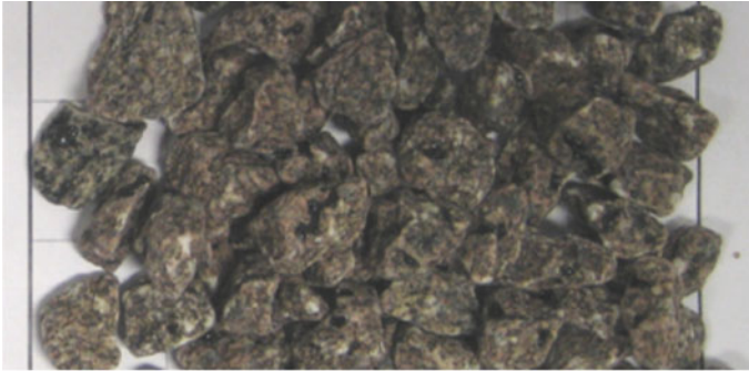
(A) Pictures of granite aggregate with PmB after 24 h from lab 1 with 5% coating
