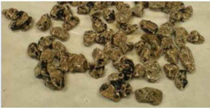
(B) Pictures of granite aggregate with PmB after 24 h from lab 4 with 20% coating
