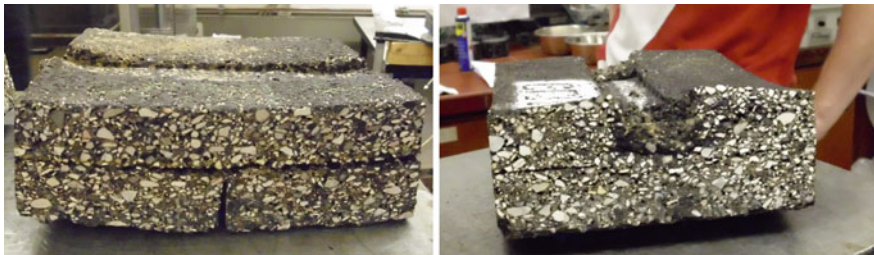
Fig. 4.49 Double-layered specimens at the end of the modified wheel tracking test
