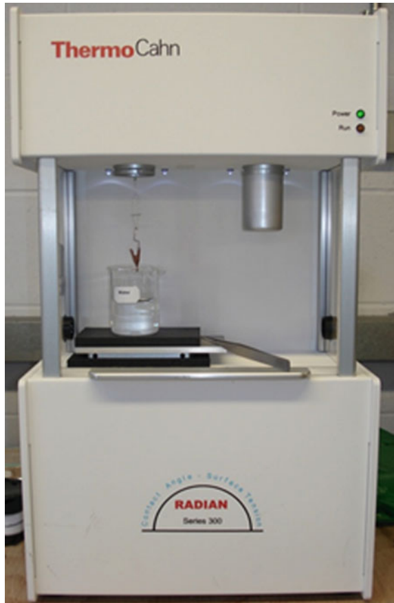
Fig. 2.18 Dynamic contact angle analyser test set-up
