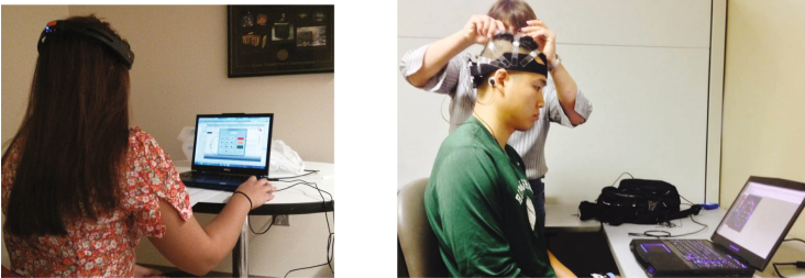
Fig. 1. (a) Experimental set up with Emotiv headset (b) Experimental set up with B-Alert headset (face masked for anonymity)
