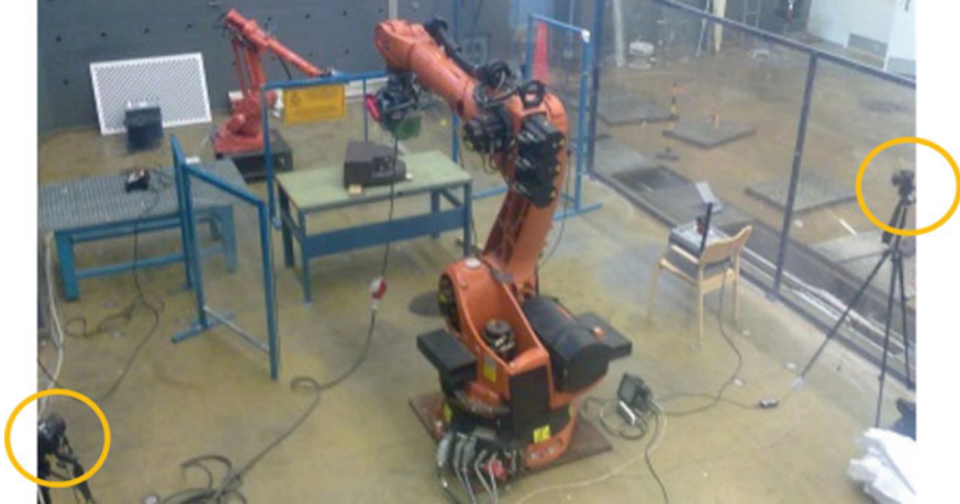
Fig. 2.10 Setup of the mold machining robot system with collaborative localizing sensors (cameras inside the orange circles)
