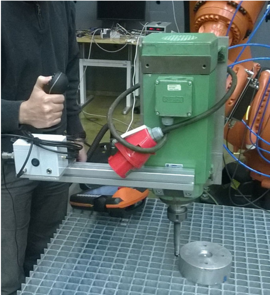
Fig. 2.2 The robot's tool is guided in contact around a stiff object (Ahola et al. 2017)
