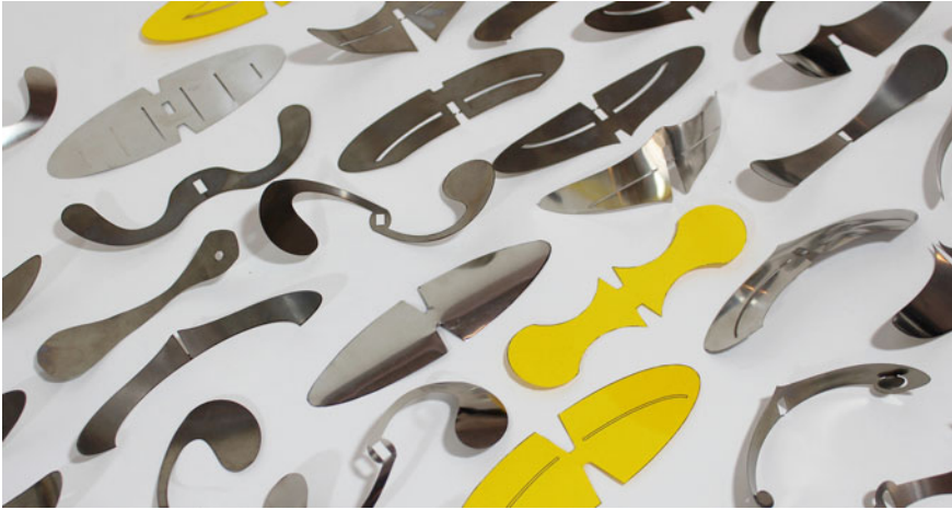
Fig. 9.3 One of the methods of programming behavior in thermobimetal is determined by the geometry of the piece so that they both flip at the correct temperature and shade at the right angle
