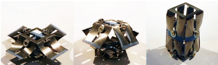
Fig. 9.8 This self-erecting box reaches over 4” tall when complete
