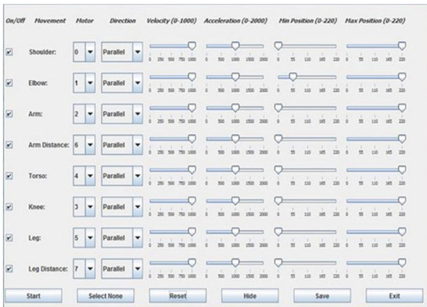
Fig. 7.2 MOVE interface to mapping possibilities. The interface lets designers map body movements to prototype movements, allowing adjustments to panel velocity, acceleration, as well as min/max positions. Configuration can also be saved here
