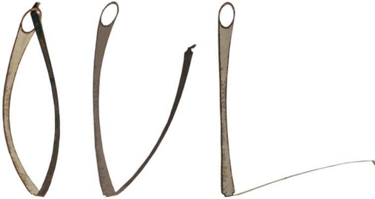
Fig. 9.7 This self-clasping link of thermobimetal is only 2" long
