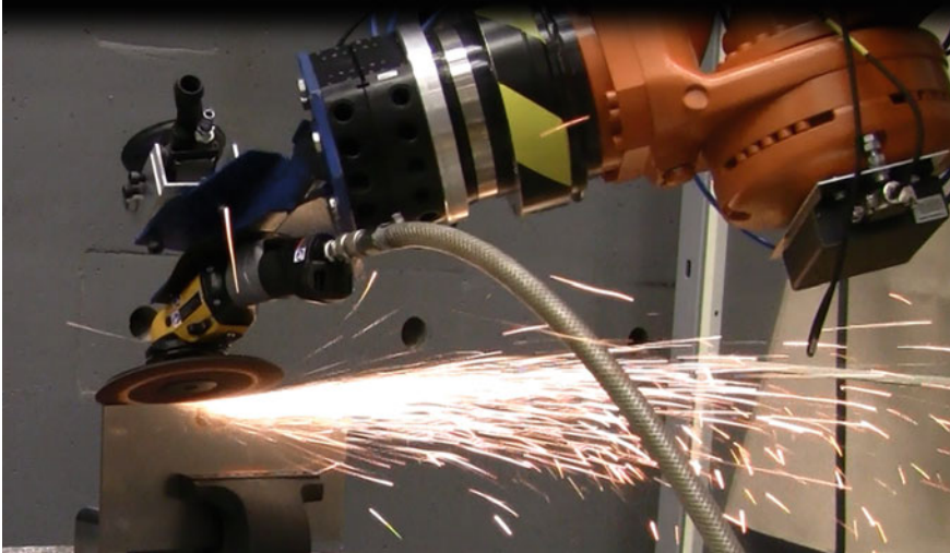
Fig. 2.6 Grinding with a force-controlled robot
