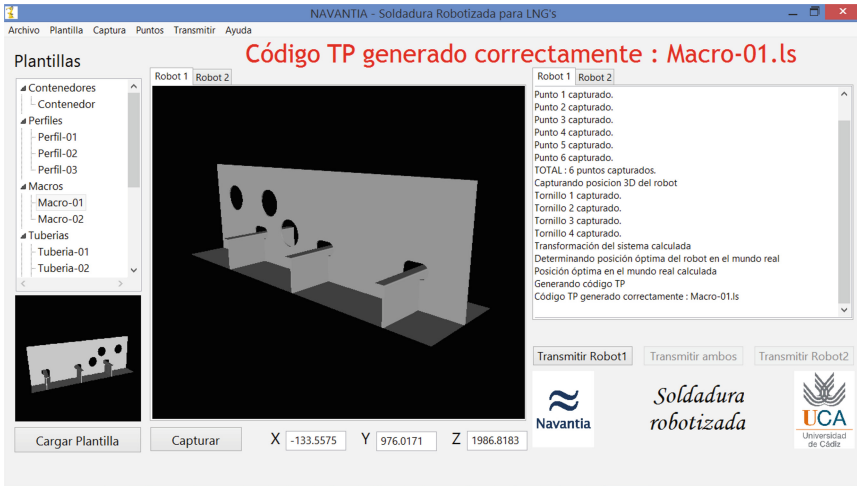
Fig. 4. Main window of the Graphical User Interface. On the left side, the template tree is shown. In the middle of the screen we may observe the chosen template in 3D. On the right hand side we may observe the message window. Three main buttons are observed: in the left side to load the template, in the center to capture coordinates using the coordinate measuring arm, and in the right side to send the resulting FANUC code to each robot.
