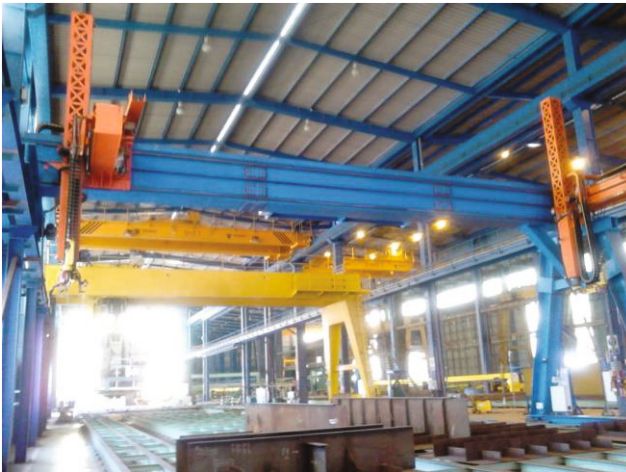
Fig. 1. Welding robotic structure: two FANUC ARCMate 100iC MIG welding robots with R-30iA controllers mounted in an 8 meters-high mobile gantry crane at Navantia company.
