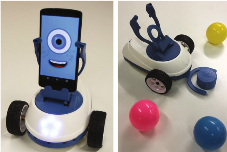
Fig. 1. The Robobo robot with the smartphone attached (left). The mobile base with a 3D printed pusher (right)
