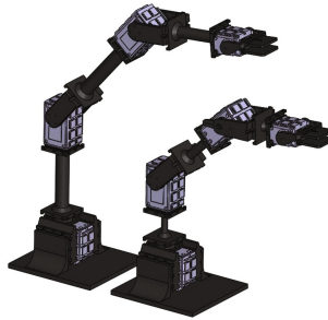
Fig. 9. Left manipulator needs two high-torque and one middle-torque actuators, while right manipulator (smaller) needs one high-torque and two medium-torque actuators.
