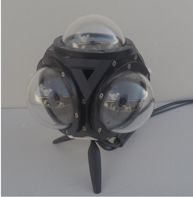
Fig. 1. Omnidirectional camera composed of five Gopro Hero 4 Black Edition.
